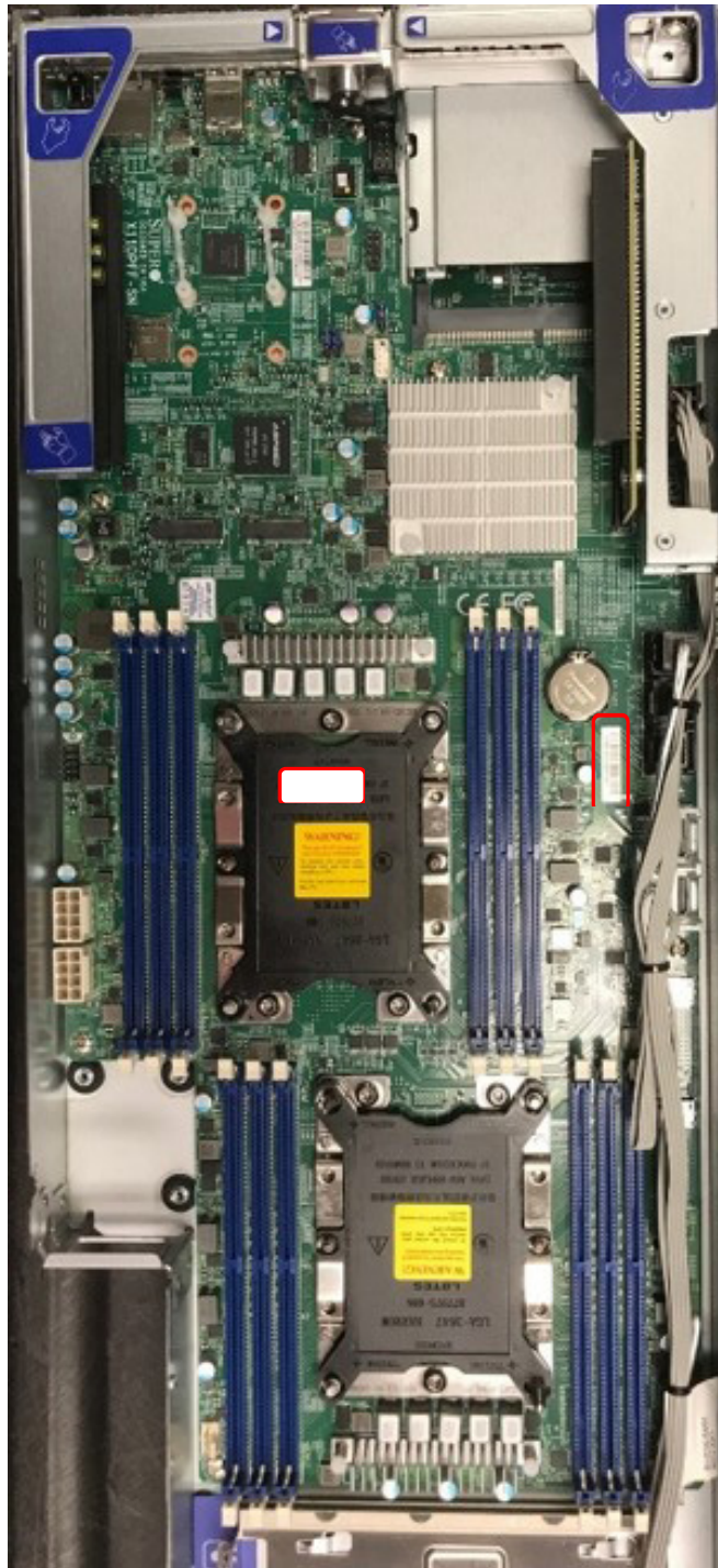
Label locations on motherboard PCB and the cover of CPU1
